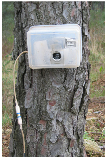
▲ Photograph 3 – Pressure plate camera trap used for lynx detection.
