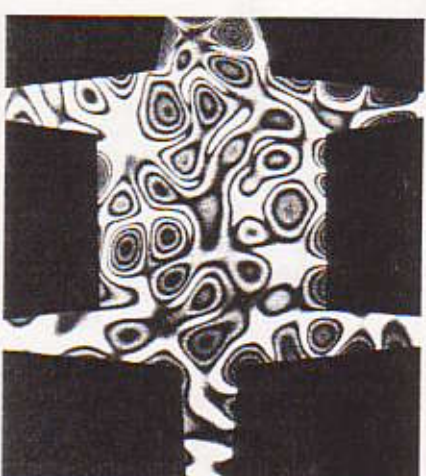
STANDING-WAVE PATTERNS generated on a thin vibrating plate resemble coat patterns and confirm the author's work. More complex patterns correspond to higher frequencies of vibration. The experiments were done by Charles M. Vest and Youren Xu.
